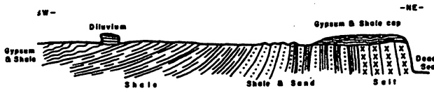
Sketch section (not to scale) through salt-mass at salt-cave, Jebel Usdum. From Wyllie (1931, p.24)
