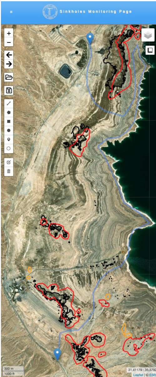
Screenshots of the field-trip trial from the monitoring system. Left: Orthophoto (ESRI) of the field-trip area. Right: LiDAR hillshaded relief map (2022). The trail is marked by light blue line. Polygons show sinkholes (black), subsidence in the past 6 months intersected by sinkholes (red) and subsidence in the past 6 months not intersected by sinkholes.
